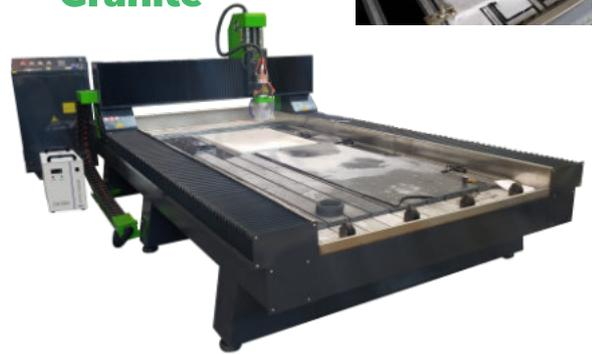
Our Stone-Tech range of stone CNC routers are perfect for any industry that has a requirement to cut and engrave into materials such as granite and marble etc.
